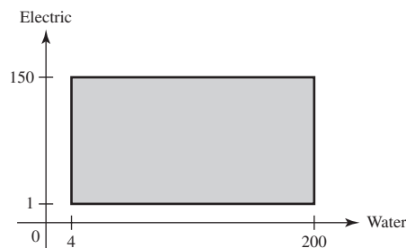
Figure 1.5 Sample space for water and electric demand in Example 1.4.5
